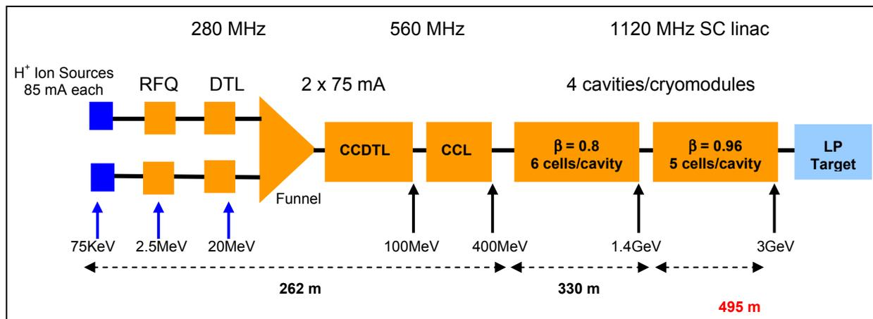
Figure 1: Alternative design layout for LP [11].
