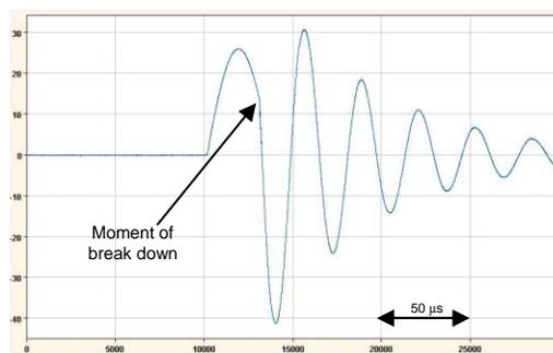
Figure 5: Measured MKB current [kA] versus time during a break down.
