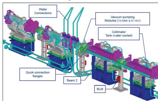
Figure 3: 3D integration in the tunnel
