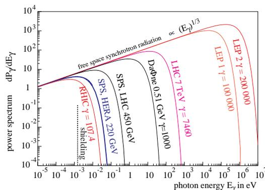
Figure 1: Calculated power spectra for synchrotron radiation.
