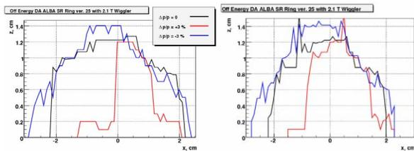
Fig.3 Off-energy DA with the SC wiggler (symplectic tracking). The right plot corresponds to the more precise optic recovering
