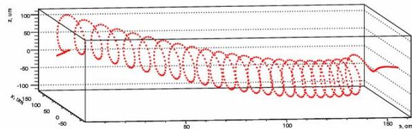
Fig.4 The beam trajectory in the HU 62 undulator
