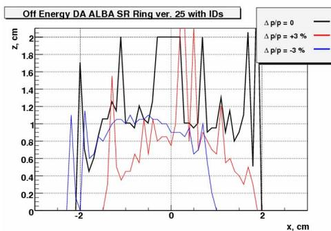
Fig.7 Off-energy dynamic aperture for the combined action of two undulators
