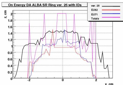
Fig.6 On-energy dynamic aperture for combined action of two undulators in comparison with their separate influence and bare lattice
