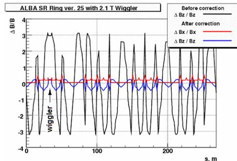
Fig.1 The ALBA-25 betatron functions beating (%) due to the SC wiggler insertion before and after correction
