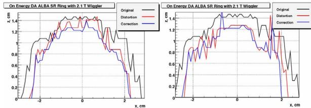
Fig.2 On-energy DA for the linear wiggler model (left) and for the symplectic tracking with the full magnetic map (right). Blue curve indicates uncorrected beta, red – corrected and black is the initial DA.
