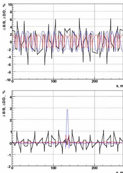
Fig.5 An example of the lattice functions distortion due to HU 62 before (upper plot) and after correction
