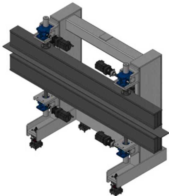
Figure 6 : Undulator frame single column design.
