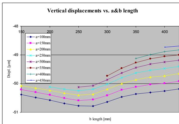
Figure 5 : Vertical frame displ. vs. A and B length.
