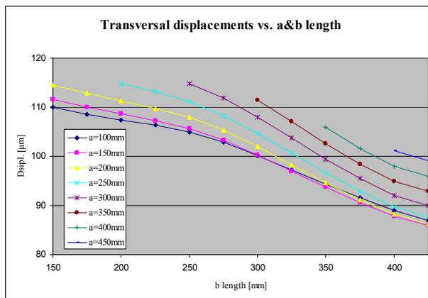
Figure 4 : Transversal frame displ. vs. A and B length.
