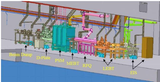
Figure 11: System layout of SARAF Phase I.
