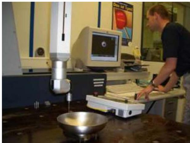
Figure 9: Half cell after deep drawing at dimension inspection
