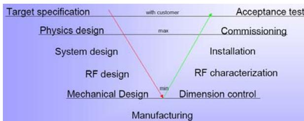
Figure 4: Project phases, from design to manufacturing and back to the system acceptance
