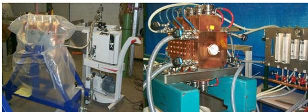
Figure 8: Leak and flow test of a CCL segment.
