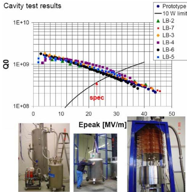
Figure 12: SARAF HWR cold tests at factory.
