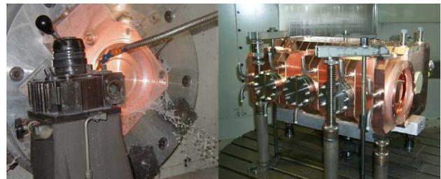
Figure 6: CCL accelerating cell during turning (left) and CCL segment after final braze on mill to get final length
