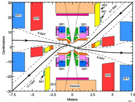
Figure 2 : PEP-II Interaction Region (IR) with head-on collisions. There are four permanent magnets within the BaBar 1.5 T solenoidal field covering +/- 2.5 m.
