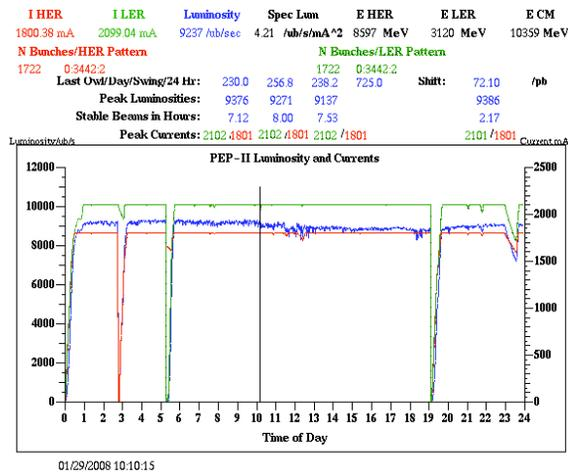
Figure 13 : Continuous injection of both PEP-II beams.
