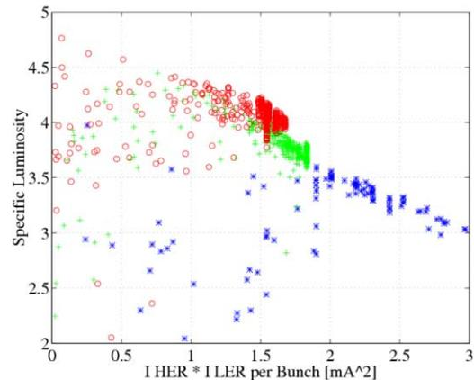
Figure 11 : Specific luminosity versus the product of the bunch currents. The specific initially rises because of dynamic beta effects and then falls due to beam-beam interaction from both primary and parasitic collisions. The parasitic beam-beam effect was only a few percent. The blue points are By-4 pattern scaled to the By-2 pattern.
