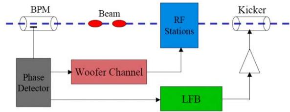
Figure 5 : Bunch-by-bunch longitudinal feedback system with an added low level (woofer) channel.
