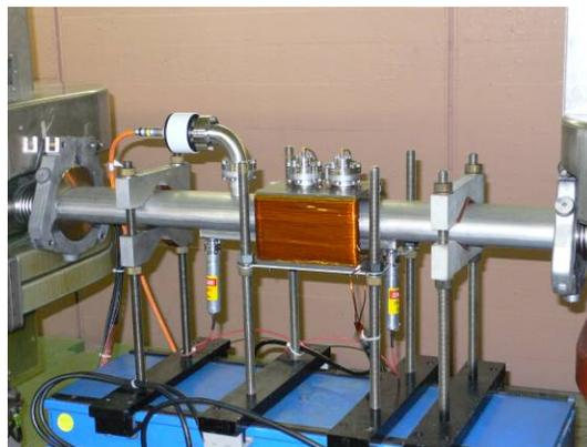
Figure 1: Picture of the PS electron cloud experiment comprising a fast vacuum diagnostic, shielded button pickups, a dipole magnet, and a clearing electrode.
