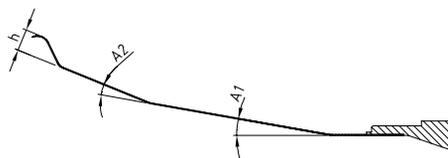
Figure 2 – Main geometrical parameters of the contact finger characterising its shape before assembly.
