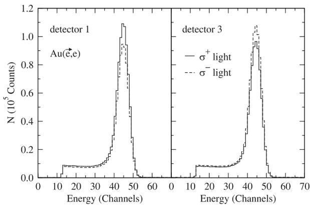
Figure 5: Measurement of Mott spectra with the two detectors of a scattering plane for reversing electron helicities. The helicity can be switched by reversing the polarization of the laser light.
