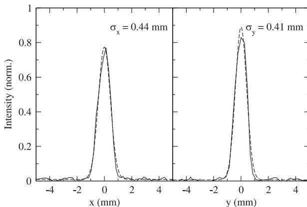
Figure 3: Measurement (solid line) of a typical beam profile. Its shape is nearly Gaussian (dashed line).
