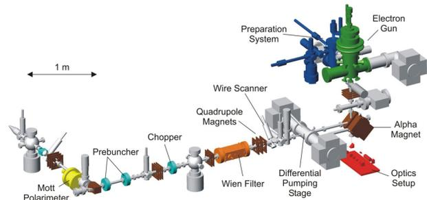
Figure 1: Schematic drawing of the teststand. A laser beam focused onto the cathode produces a polarized electron beam by photoemission. After pre-acceleration to 100 keV it is injected into the horizontal test beamline where its properties can be studied. The chopper and prebuncher system is not yet installed.
