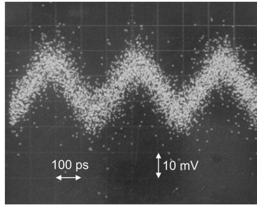
Figure 4: Measurement of the time structure. The period of approx. 330 ps matches with the 3 GHz S-DALINAC time structure.
