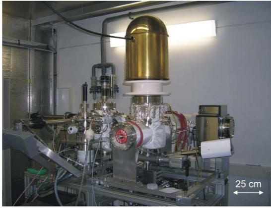
Figure 2: Photograph of the electron source (center) and the preparation system (left).
