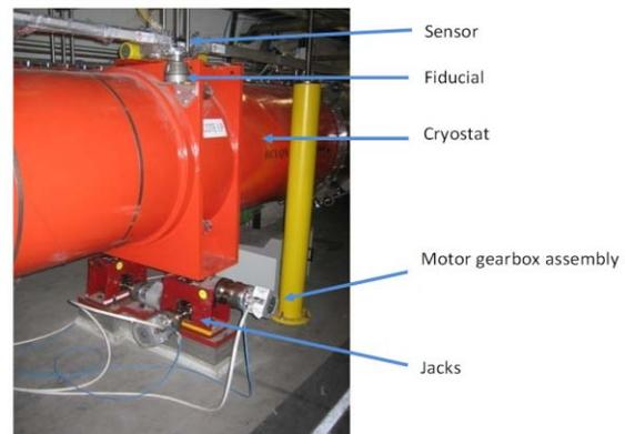
Figure 2: Complete assembly of equipment.
