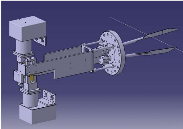
Figure 5: Mechanical drawing of the vertical scraper.
