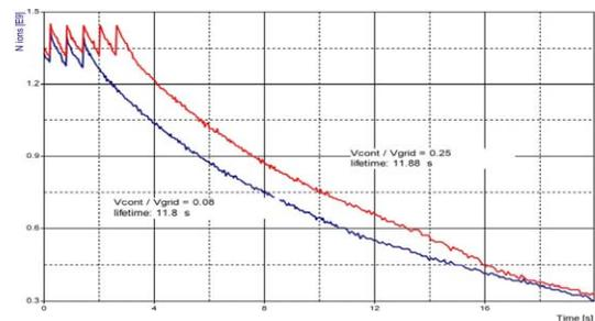
Figure 7: Example of a beam lifetime measurement.
