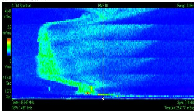
Figure 2: Longitudinal Schottky spectrum measured on the Agilent N9020A vector signal analyser at the 100<sup>th</sup> harmonic during five LEIR injection-cooling sequences.
