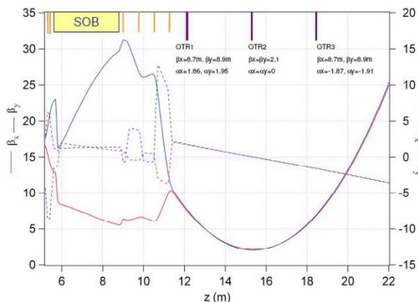
Figure 3: evolution of the betatron functions in the low energy diagnostic section.
