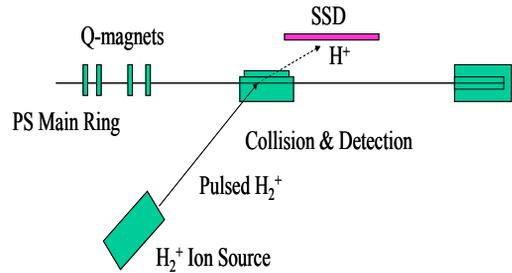
Figure 2: Single path collision scheme.
