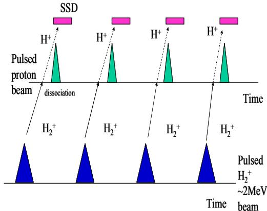
Figure 1: Principle of extinction monitor and micro structure of beam.
