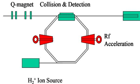
Figure 3: Storage and acceleration ring of  $H_2^+$  ion and detection section of dissociated atoms.
