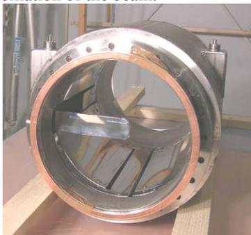
Figure 6: SPUC prototype. (Before the orifice is drilled in the scraper.)
