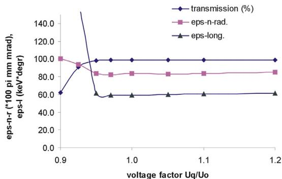
Figure 6: Simulation of beam dynamics versus RFQ field level
