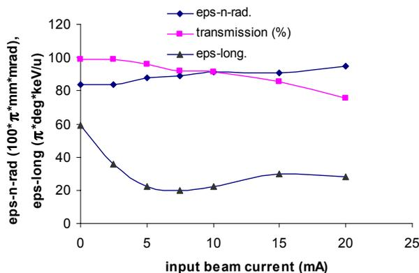
Figure 7: Simulation of beam dynamics versus input beam current
