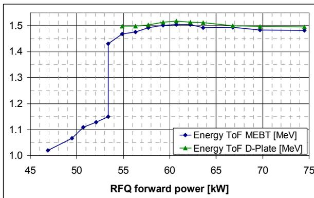
Figure 3: Energy measurements by ToF method versus RFQ power
