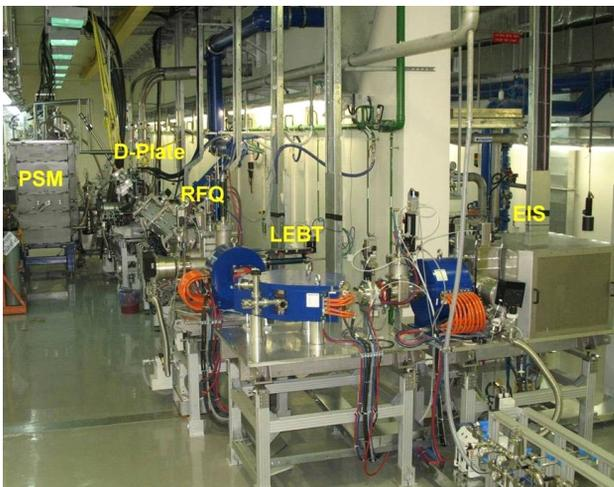
Figure 1: SARAF accelerator Phase 1 installed in the tunnel. From right to left: ECR Ion Source, Low Energy Beam Transport (LEBT), RFQ, Diagnostic-Plate and Prototype Superconducting Module (beside beam line)
