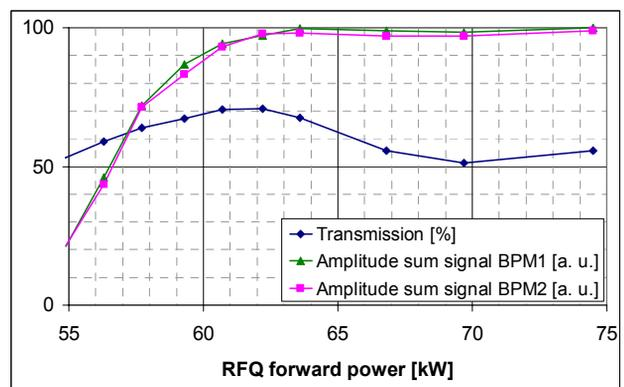
Figure 2: Transmission through the RFQ and amplitude of MEBT-BPM sum signals versus RFQ power
