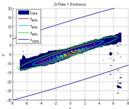
Figure 5: Transversal emittance measurements in the D-Plate by slit and wire method
