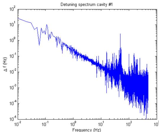
Figure 8: Typical microphonics detuning spectrum\*
