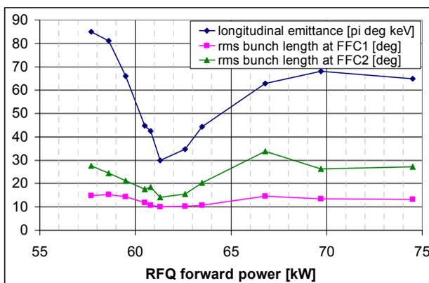
Figure 4: Bunch length measurements behind the RFQ versus RFQ power for determination of longitudinal emittance
