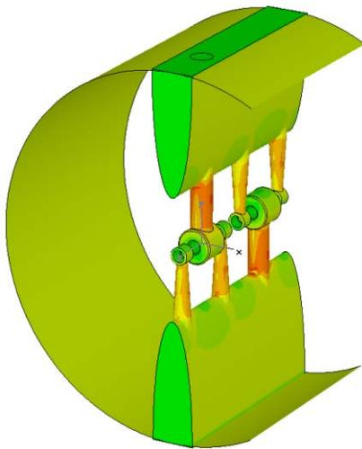
Figure 3: Surface current magnitude in the modified IH1-3 structure (the cavity wall is partially cut).
