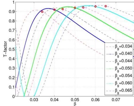
Figure 2: Transit-time factor of different IH structures (defined by  $\beta_g$ ) versus beam velocity  $\beta$ .
