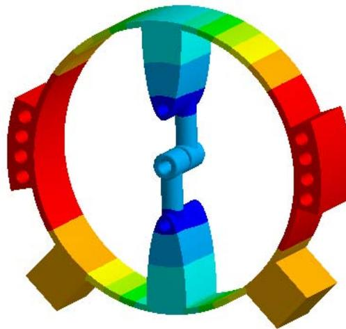
Figure 4: Temperature distribution in regular IH structure.
