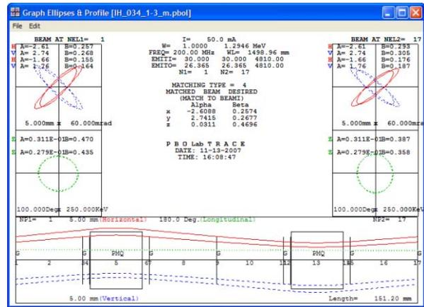
Figure 1: Beam matching results for IH1-3 at  $\beta_g = 0.034$ .
