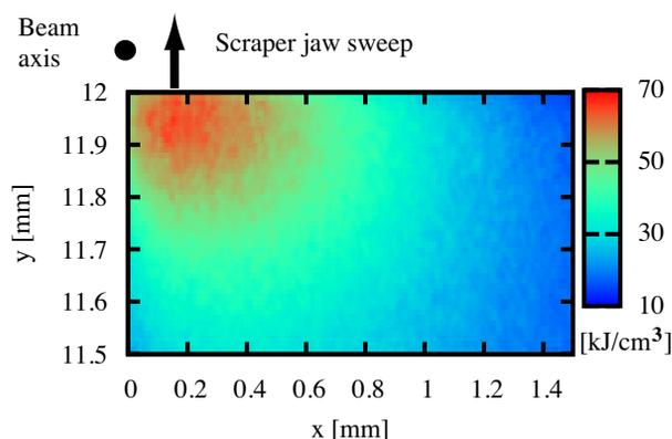
Figure 6: Energy deposit density for a faster and thinner copper scraper jaw. Note that the heat load spreads out more than in Figure 5.
