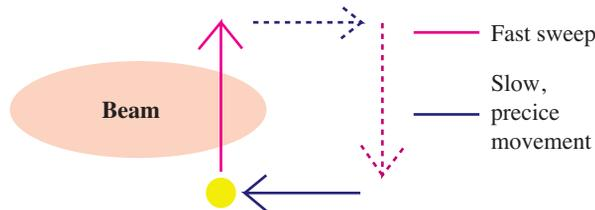
Figure 2: Schematic view of the scraper jaw's movement relative to the beam. Note that the scrapers always sweep through the beam quickly, with velocity  $v = 20$  cm/s. Only the horizontal scraper is shown here.
