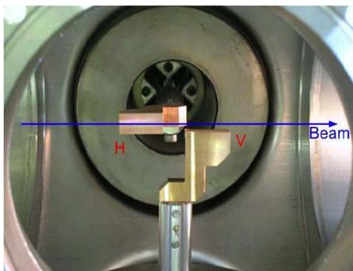
Figure 1: The two scraper jaws, horizontal and vertical.
