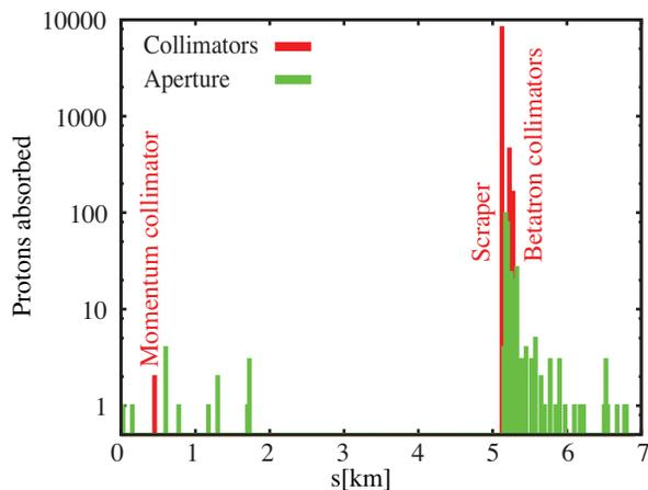
Figure 3: Simulated proton losses around the SPS ring. Note that the scrapers absorb over 80% of the protons, while collimators and aperture absorb roughly 10% each. A beam halo of  $10^4$  protons at  $4\sigma$  was simulated.
