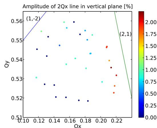
Figure 4: Amplitude of the skew sextupolar resonance (2,1) through the amplitude of the spectral line(2,0)<sub>v</sub> versus tunes. The amplitude increases as the resonance is approached.
