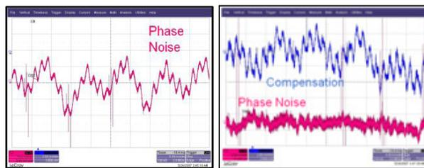
Figure 8: Klystron Phase Ripple (10mV/deg): Left Polar loop off, scale 10mV/div. Right: Loop on, scale 2mV/div.
