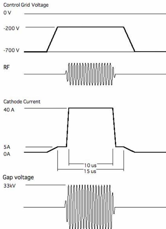
Fig. 2: Typical timing chart in case of PRISM. For the 6-cell ring, RF on time is extended to 30  $\mu$ s.
