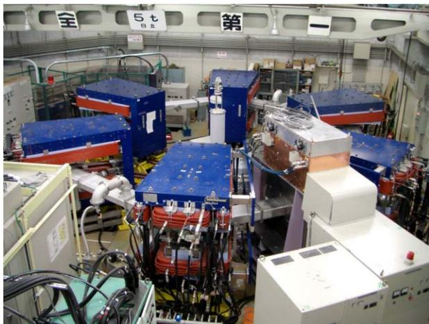
Fig. 1: 6-cell FFAG ring to demonstrate bunch rotation. A MA cavity system is also shown. The amplifier is located on top of the cavity. An anode power supply is set beside of cavity. The anode voltage is delivered to the amplifier by a bus bar.
