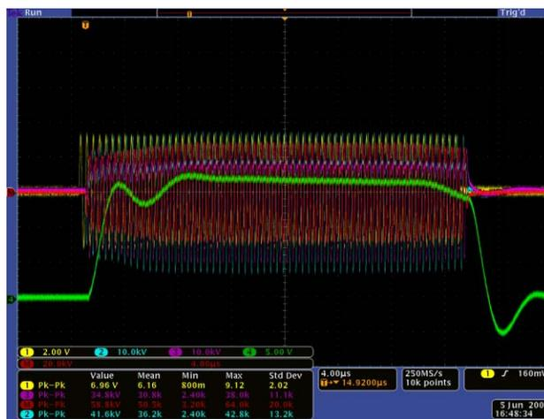
Fig. 3: Typical gap voltage for 100 Hz repetition. The duration was extended to 30  $\mu$ s. The timing has not yet been adjusted. Yellow and red lines mean input and gap voltages, respectively. The green line shows the anode current.
