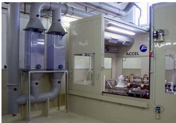
Figure 6: Completely installed and commissioned EP plant at ACCEL. In this plant every day at least one cavity can be treated.
