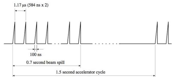
Figure 2: Required time structure of proton beam.
