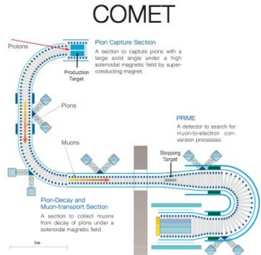
Figure 1: Schematic layout of the muon beam line and detector system of COMET experiment.
