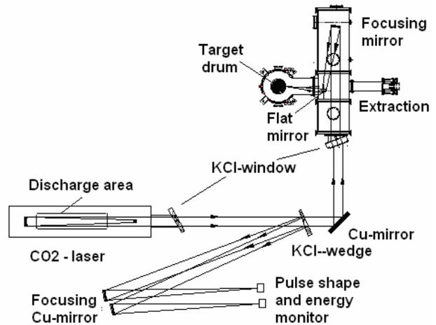
Figure 1: The 100J CO<sub>2</sub>-laser ion source optical scheme.
