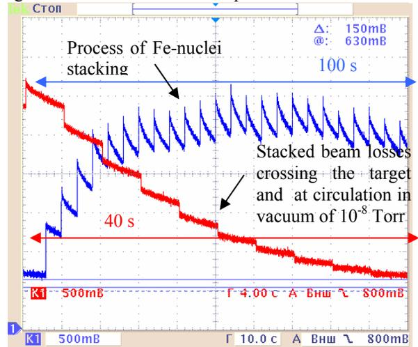
Figure 7: Stacking of  $\text{Fe}^{26+}$ -nuclei in the U-10 ring.
