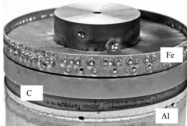
Figure 5: The LIS target drum after long time operation with Fe- Al- and C- beam generation.
