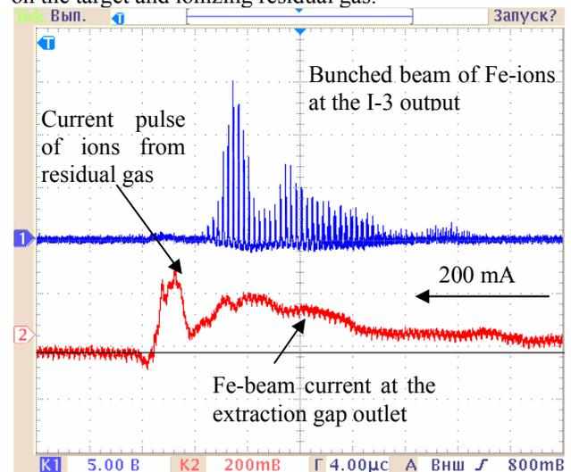
Figure 2: Signals of Fe-ion beam generated in LIS.
