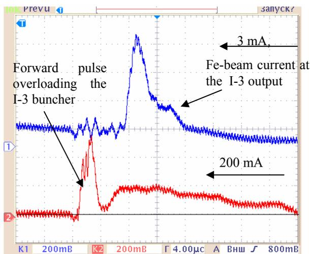
Figure 4: Current signals of total Fe-beam at the LIS extraction gap outlet and  $Fe^{16+}$ -beam of 64 MeV at the I-3 linac output.
