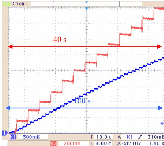
Figure 6: The stairs of  $\text{C}^{6+}$ -beam stacking in the U10 ring.
