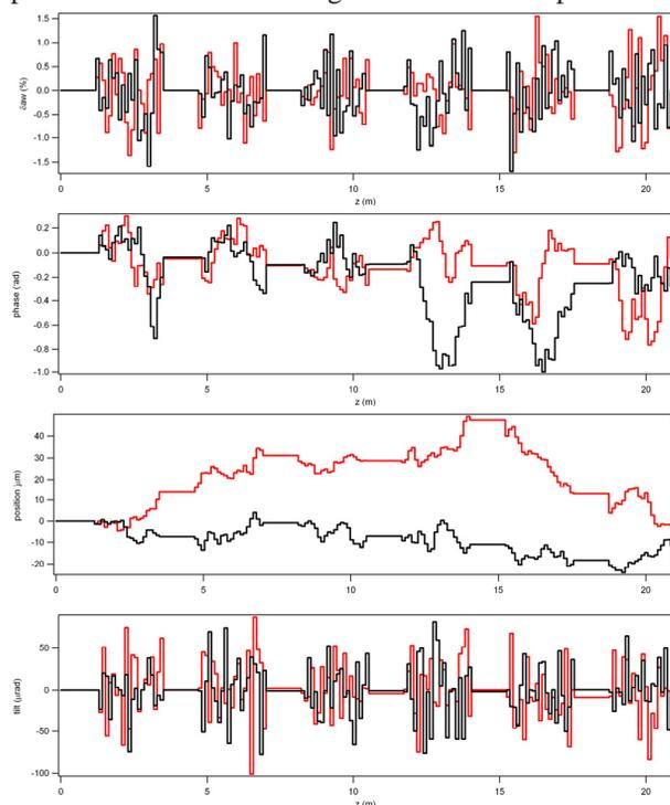
Figure 4: Two examples of the evolution of the undulator error AW along the radiator (a) and their effect on the electron beam in terms of phase (b) position (c) and tilt (d) errors.
