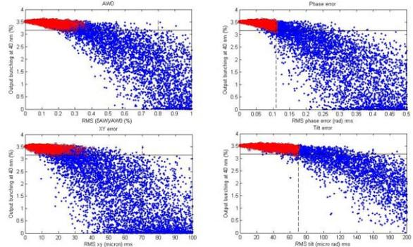
Figure 3: Reported data show how filtering the data in the 4D parameter space allow to relax the requirements for the undulator. In figure red dots refer to data corresponding to undulator error configuration whose errors in terms of AW phase, position and tilt are within the selected limits also reported in figures by vertical dashed lines.
