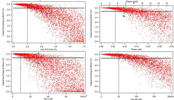
Figure 1: Produced bunching at 40nm at the exit of the dispersive section as a function of the rms AW error (a), rms phase error (b), rms position error (c) and rms tilt error (d). The green triangle and blue square refer to two AW error distributions with similar rms phase error (b). Corresponding evolution of the electron beam's phase, position and tilt along the undulator are reported in Fig.2 (b,c,d).
