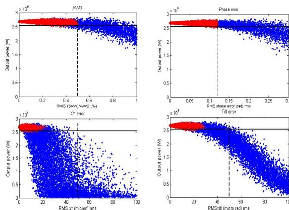
Figure 5: Reported data show how filtering the data in the 4D parameter space allow to relax the requirements for the radiator. Red dots refer to data corresponding to undulator error configuration whose errors in terms of rms AW, phase, position and tilt are within the selected limits (represented by the vertical dashed lines).
