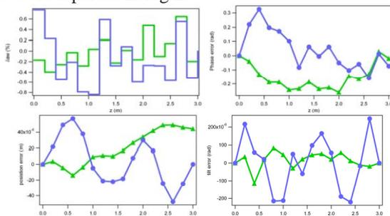
Figure 2: Evolution of AW along the modulator and corresponding position, phase and tilt errors for the electron beam passing through the undulator. Corresponding performance in terms of produced bunching for these two cases are reported in Fig.1 with equivalent colors and symbols.
