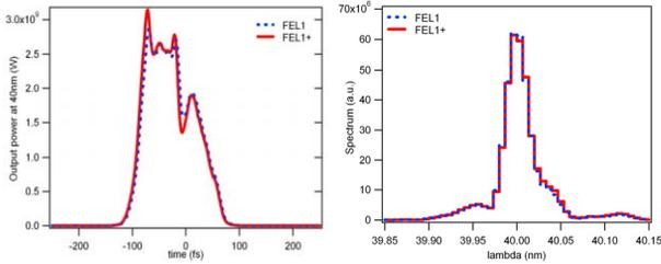
Figure 2: Output temporal (left) and spectrum (right) profiles of FEL1<sup>+</sup> (continuous line) and FEL1 (dotted line) at 40 nm. In both cases, six radiator sections have been considered.
