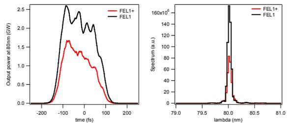
Figure 6: Left: power profile at the exit of FEL1 (black line) and FEL1<sup>+</sup> (red line) tuned at 80 nm. Right: Corresponding spectrum profiles. In both cases only three radiator sections have been used.
