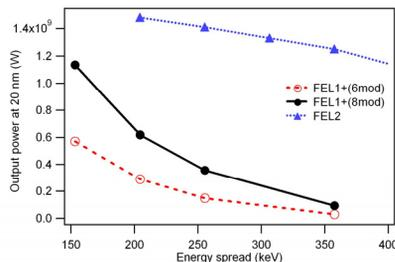
Figure 5: FEL1<sup>+</sup> (continuous (8 sections) and dashed (6 section) lines), and FEL2 (dotted line) output power at 20 nm as a function of the electron-beam energy spread.
