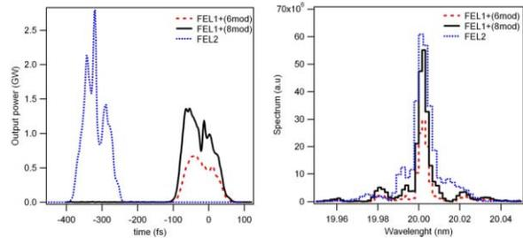
Figure 4: Output temporal (left) and spectrum (right) profiles of FEL-1<sup>+</sup> (dashed: 6 radiator sections, continuous: 8 radiator sections) and FEL-2 (dotted line: eight radiator sections) at 20 nm.
