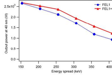
Figure 3: Expected power from FEL1<sup>+</sup> (continuous line) and FEL1 (dashed line) at 40 nm as a function of the electron-beam energy spread.
