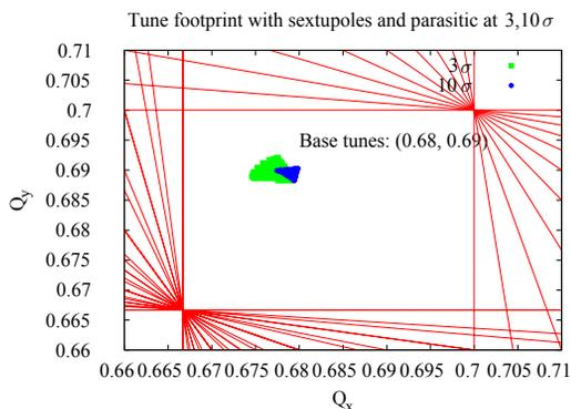
Figure 3: Tune footprints with beam separations at 3 (in green) and 10  $\sigma$  (in blue). At 10 $\sigma$ , the beam-beam interaction has little impact on the tune spread, it is almost entirely due to the sextupoles.
