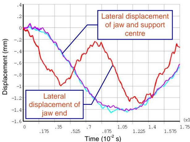
Figure 7 Time history of deflection of the centre and the ends of the C/C jaw for the series secondary collimator
