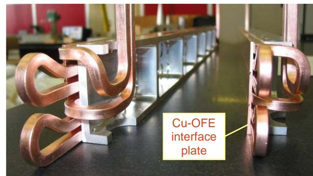
Figure 2: Collimator prototype metal supports ( $\sim 1\text{m}$  long), showing the stainless steel support bar, the cooling pipes and the 3 mm-thick interface Cu-OFE plate
