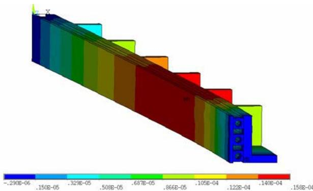
Figure 6 Residual deflection (maximum 16  $\mu\text{m}$ ) of the modified series metal support (Cu-Ni pipes, Glidcop support beam and thin plate)
