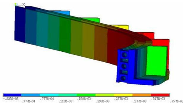
Figure 5 Residual deflection of the prototype metal support (maximum 357μm)
