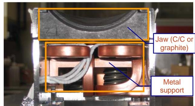
Figure 1 Front view of the collimator jaw assembly showing the carbon jaw and the metal support
