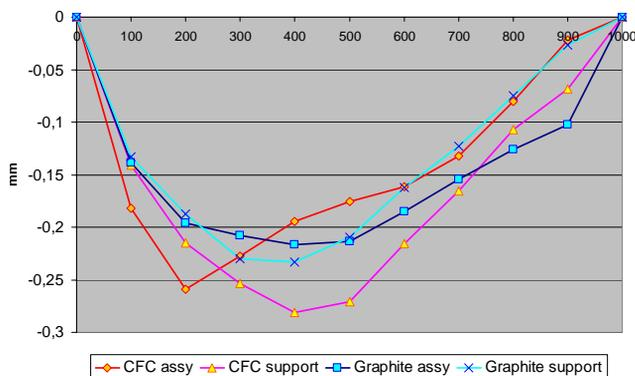
Figure 3: Permanent deformation of the jaw assemblies and metal supports as a function of the length (1000mm)
