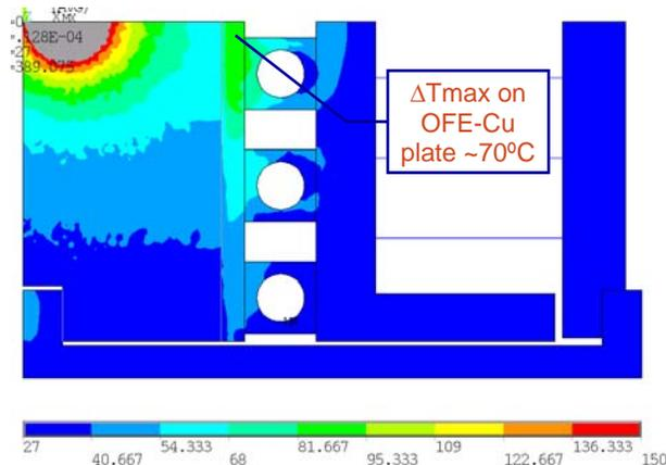
Figure 4: Temperature distribution after the thermal shock at the hottest cross-section of the jaw assembly
