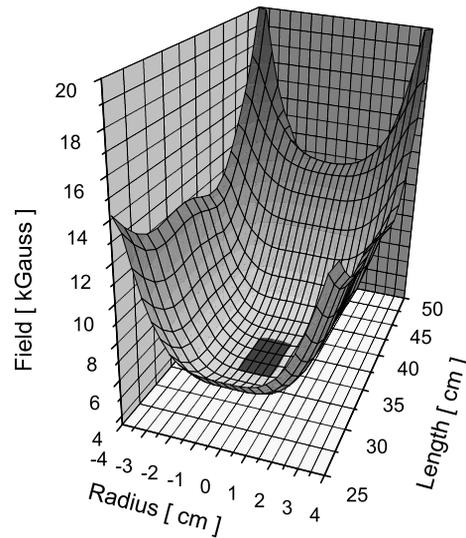
Fig. 2: Three-dimensional view of magnetic field distribution. The dark area in the centre corresponds to the enlarged resonance zone.
