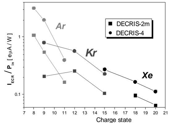
Fig. 5: Comparison of efficiency of ion sources.
