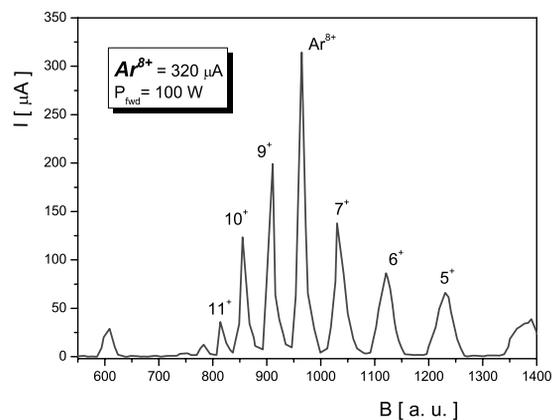
Fig. 3: Argon spectra optimized to Ar<sup>8+</sup>.
