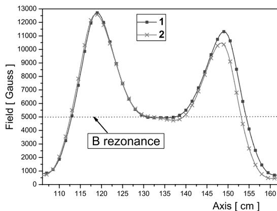
Fig. 1: Magnetic field distribution on the axis DECRIS-4.
