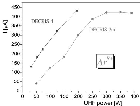
Fig. 4: Comparison of  $\text{Ar}^{8+}$  ion yields from the DECRIS-4 and DECRIS-2m ion sources.
