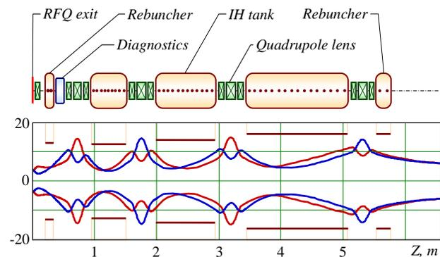
Figure 1. Accelerating structure layout and transverse beam envelopes at full current
