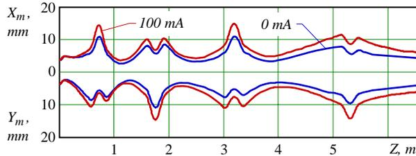
Figure 2. Transverse envelopes for 98% of particles at full current and at zero current
