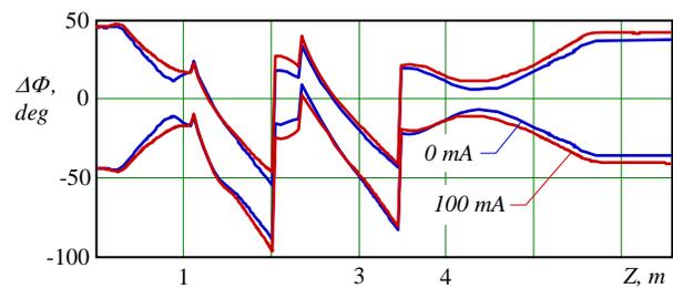
Figure 4. Phase envelopes for 98% of particles along IH structure
