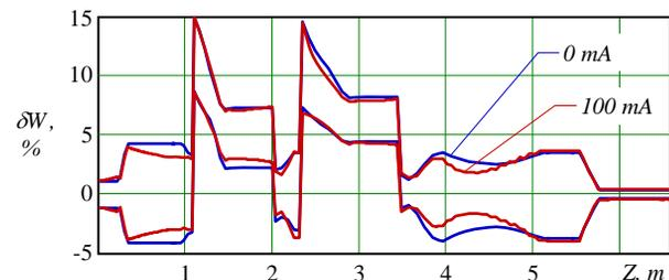
Figure 5. Energy spread for 98% of particle along IH structure
