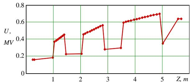
Figure 8. Effective gap voltages along IH structure
