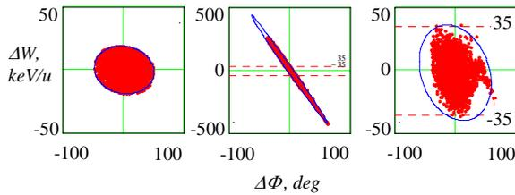
Figure 6. Longitudinal emittance at the RFQ exit, at the exit of tank 3 and behind of the final external buncher
