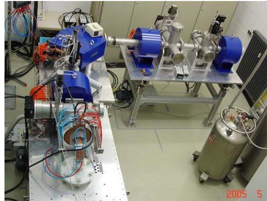
Figure 1: ECR Ion Source with LEPT in the ACCEL test facility.
