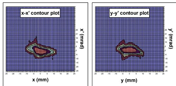
Figure 3: Beam emittance measurement ( $\epsilon_{\text{norm,rms,100\%}} = 0.15 \pi$  mm mrad at 5 mA H<sup>+</sup>).
