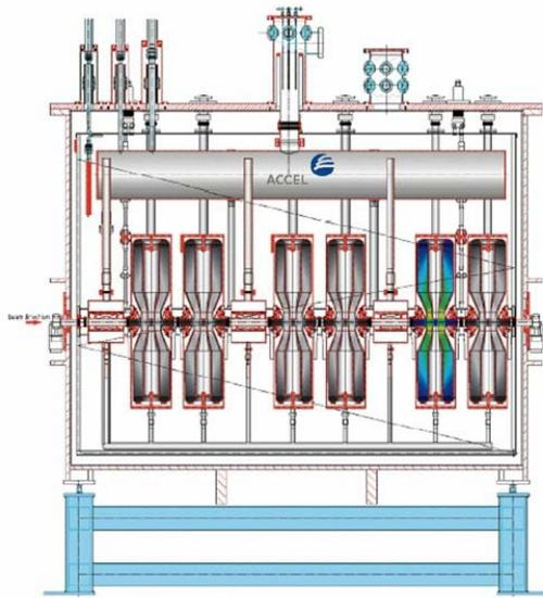
Figure 4: Prototype superconducting module containing six superconducting half wave resonators ( $\beta=0.09$ ) and three superconducting solenoids.
