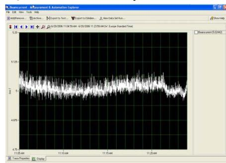
Figure 2: Beam stability measurement ( $\pm 1\%$  over one hour at 5 mA H<sup>+</sup>).
