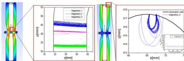
Figure 7: Two kind of stable trajectories detected inside the prototype resonator, type 1 at the high electric field region and type 2 at the high magnetic field region.
