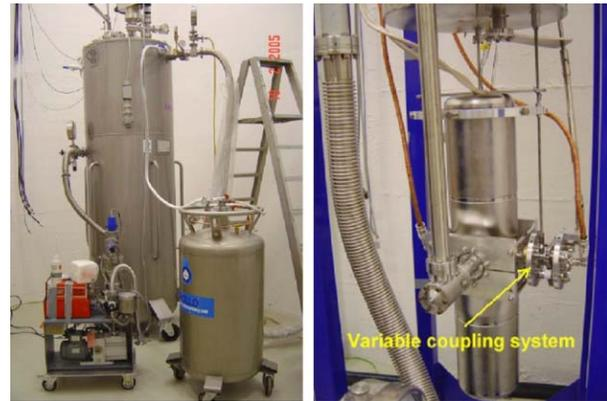
Figure 5: Vertical test facility at ACCEL. The cryostat (left) is filled with helium out of dewars and pre-cooled with LN<sub>2</sub>. The superconducting half-wave resonator is equipped with a variable input coupler for the vertical test (bottom).
