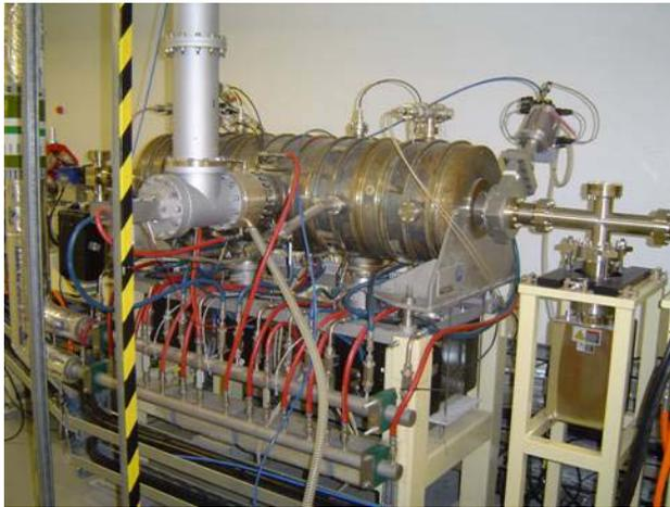
Figure 1: Booster cavity.
