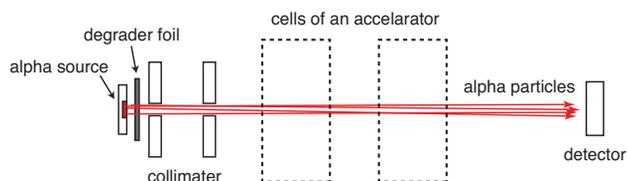
Figure 1: Schematic experimental setup.
