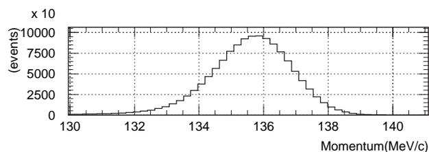
Figure 2: Momentum distribution of emitted and degraded alpha particles estimated using Geant3.21 [4]. The emission energy and thickness of the Al foil were assumed as  $5.486 \text{ MeV}$  and  $15.7 \mu\text{m}$  respectively.
