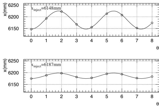
Figure 4: Betatron Oscillation behavior for two different starting positions injection radius; 6148mm (upper) and 6187mm (lower). The lower simulation shows that the injection radius is close to the equilibrium radial position. The numbers indicated on the horizontal axis show the azimuthal location of the detector.
