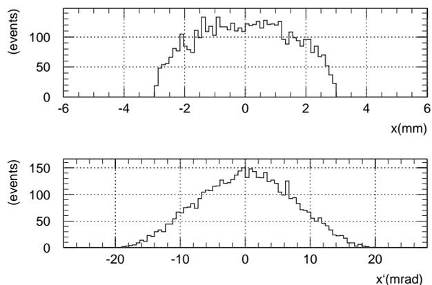
Figure 3: Simulation results of spatial and angular distribution of alpha particles after collimators which have  $D = 6 \text{ mm}$ ,  $h = 6 \text{ mm}$ ,  $L = 300 \text{ mm}$ .
