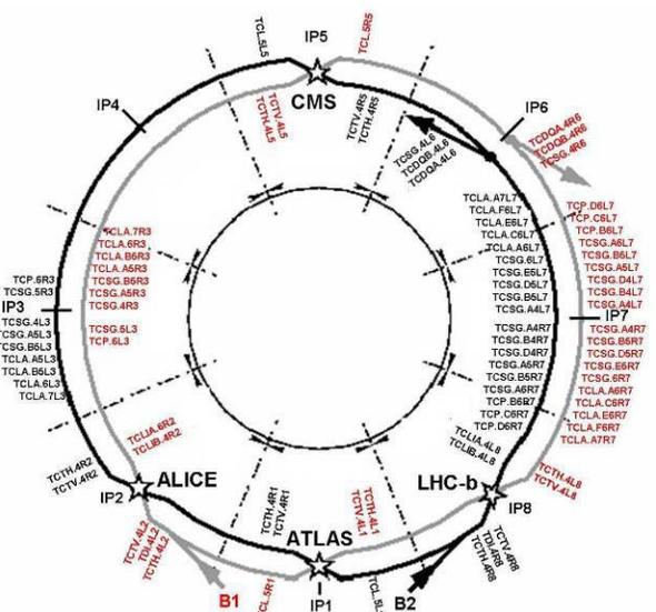
Figure 2: Layout for LHC collimation during phase 1. Red labels are beam 1 collimators; black labels beam 2).
