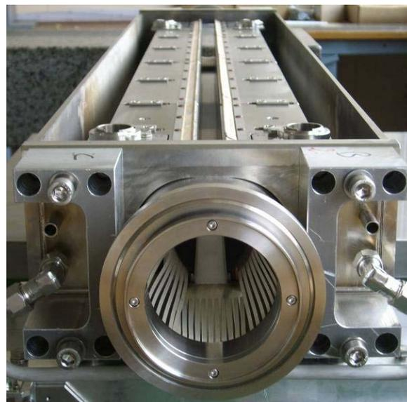
Figure 4: A view of a series TCS collimator during production. Both jaws and RF contacts have been mounted.
