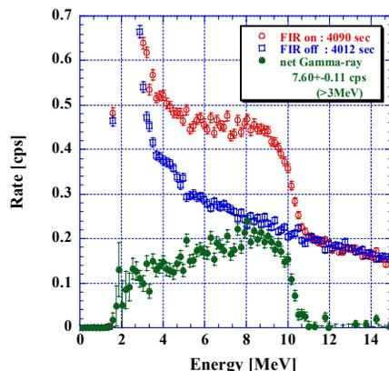
Figure 5: Measured energy spectrum of LCS MeV photons.
