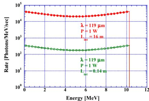
Figure 6: Comparison BL05SS with BL38B2 by calculated LCS MeV photons spectra.
