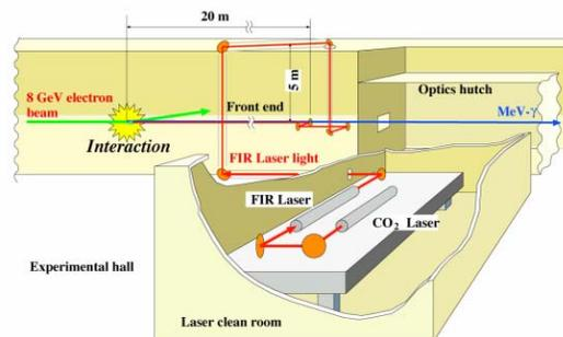
Figure 2: Laser transportation system with hollow dielectric waveguides and corner mirrors.
