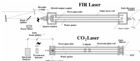
Figure 1: Schematic view of FIR laser system.
