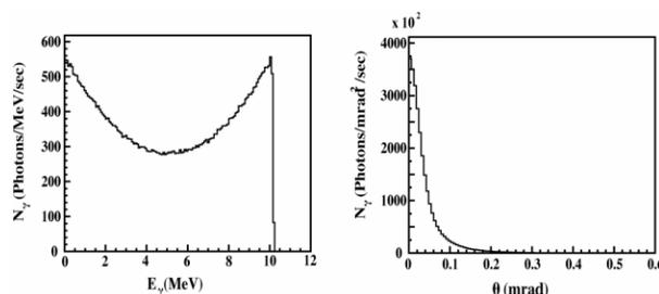
Figure 3: Calculated energy and angular distributions of LCS MeV photons by Monte-Carlo simulation.
