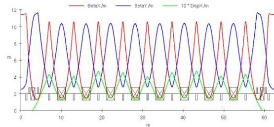
Figure 1: Machine functions along one quarter of the booster.
