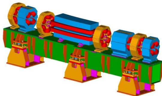
Figure 4: CAD drawing of one of the girder for ALBA.
