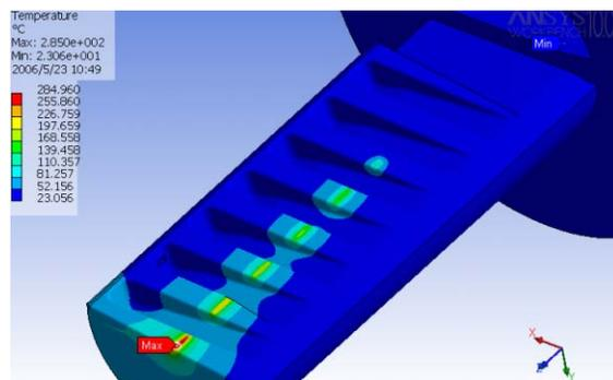
Figure 3: The FEA results for the temperature map for the most critical absorber (type 4), made of Glidcop.
