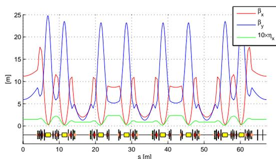
Figure 2: Machine functions along one superperiod of the storage ring.
