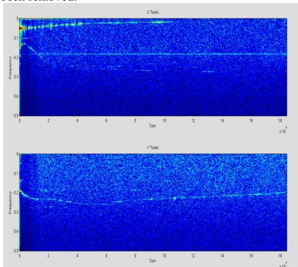
Figure 2: Horizontal and vertical tune during ramping on a turn by turn basis. (the line at 0.18 is an artefact and can be ignored)
