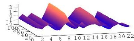
Figure 1: Booster ramp orbit, horizontal scale: BPM number around circumference, Vertical scale: orbit deviation mms and depth scale: time in 0-100ms range. Upper trace horizontal, Lower trace vertical.
