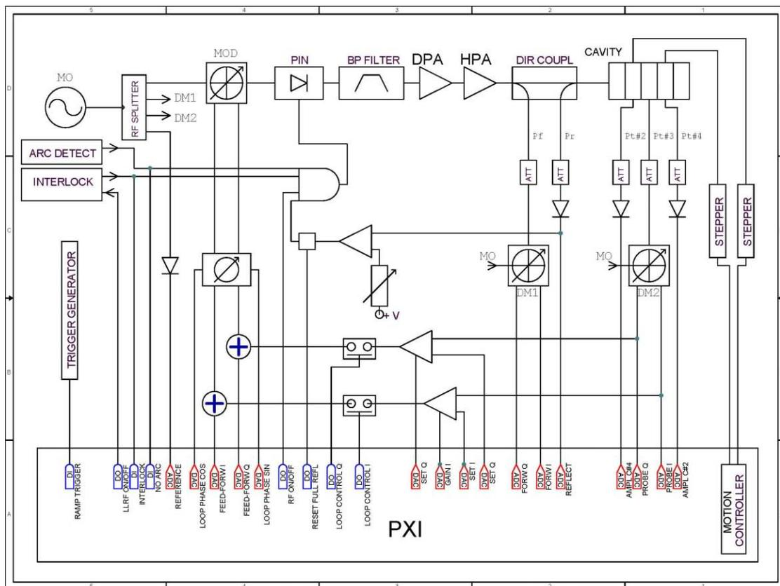
Figure 4: ASP booster LLRF diagram.
