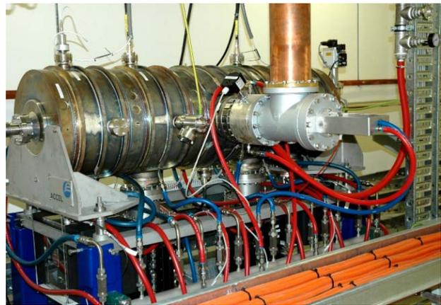
Figure 3: ASP Booster Cavity after installation.
