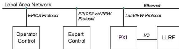
Figure 5: Booster LLRF Communication Network.
