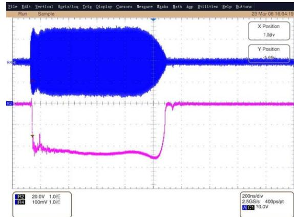
Figure 3: Beam current of MEG with hydrogen terminated CVD diamond cathode (bottom) and RF power delivered to the cavity (top), both on a 1µs / div. time scale.
