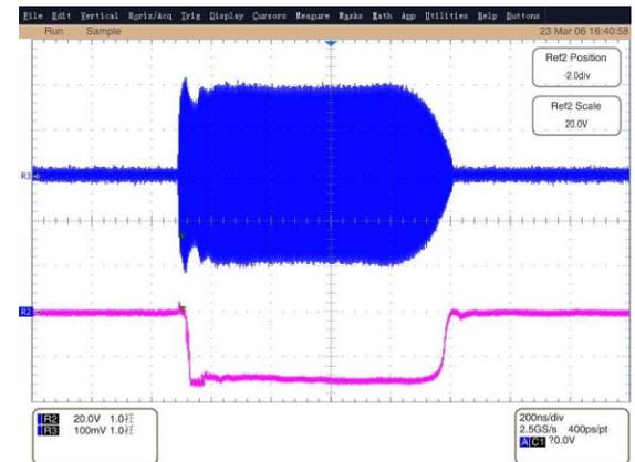
Figure 4: Beam current of MEG with CsI terminated CVD diamond cathode (bottom) and RF power delivered to the cavity (top), both on a 1µs / div. time scale.
