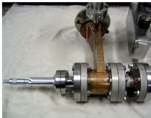
Figure 1: Photograph of the Multipactor Electron Gun.
