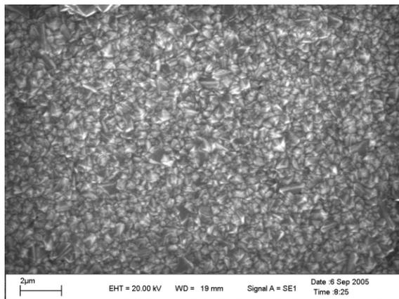
Figure 2: SEM image of the CVD diamond film.
