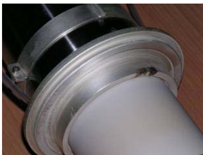
Figure 2: Evidence of arcing around the output ceramic on an IOT.
