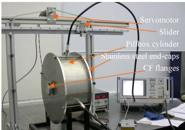
Figure 4: Bead-pull experiment setup in Imperial College London
