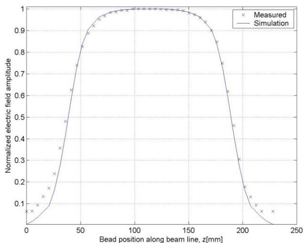
Figure 5: Electric-field distribution along beam-axis for simple pillbox cavity
