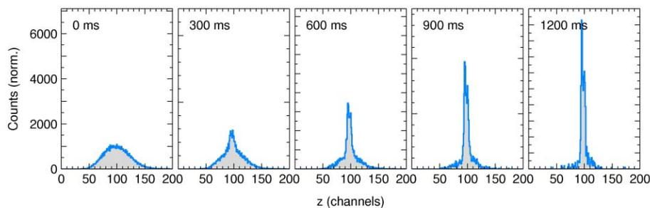
Figure 3: Transverse beam profiles during electron cooling of  $H^-$  ions. The full horizontal scale of 200 channels corresponds to 40 mm, and the time interval between the profiles is 300 ms.
