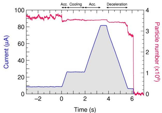
Figure 5: Proton beam current and particle number as in fig. 4 but at higher beam intensity.
