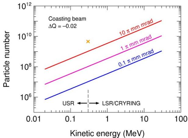
Figure 2: Space charge limit in LSR/CRYRING and USR for a coasting beam with  $\Delta Q = -0.02$ . The cross represents the maximum number of protons that could be stored in CRYRING.
