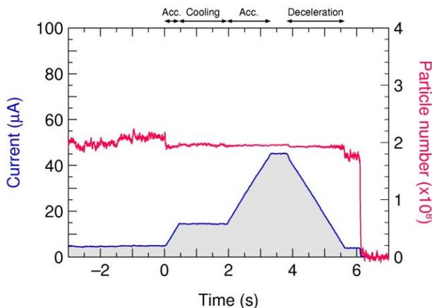
Figure 4: Proton beam current and particle number as functions of time during acceleration and deceleration.
