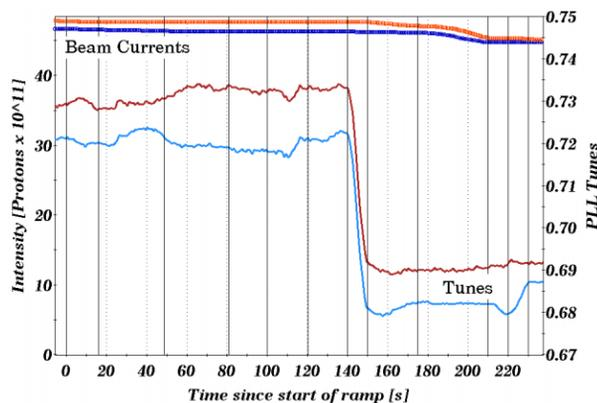
Figure 5: A typical Run-5 polarized proton acceleration ramp, showing no beam loss as tunes are moved from injection to store values.
