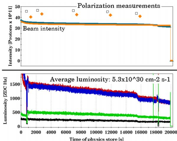
Figure 4: A typical Run-5 polarized proton store, with 45 bunches of  $0.8 \times 10^{11}$  and 40–45% beam polarizations. Polarization and beam intensity are roughly constant throughout the store; luminosity degrades due to transverse emittance growth driven by beam-beam forces.
