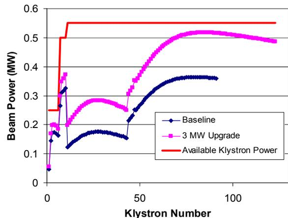
Figure 1: Beam power requirements per klystron in the baseline and 3 MW upgrade scenarios. Note that for the first 10 klystrons, the power values are divided by ten.
