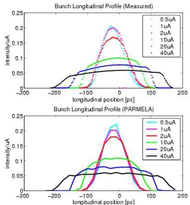
Figure 2. Longitudinal density profiles for a beam with 31 MHz repetition rate at the chopper slit. Wien filter is off. Top panel, measured. Bottom panel, simulations.
