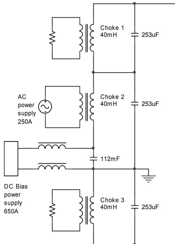
Fig. 4. Model choke test circuit.
