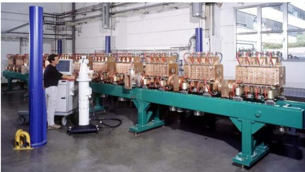
Figure 3: Alignment of 12 CCL-Segments for SNS during assembly before delivery.
