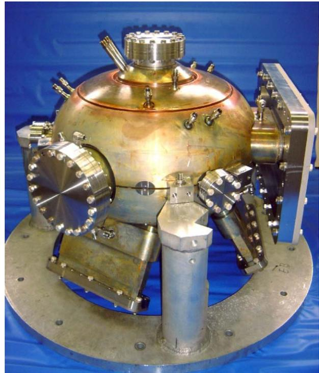
Figure 1: PEP II cavity ready for delivery
