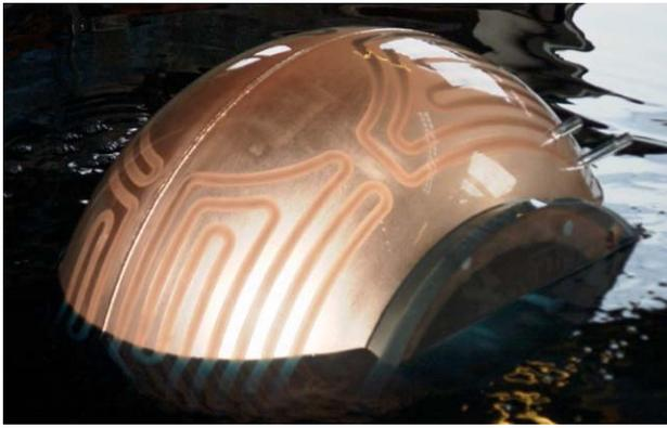
Figure 2: PEP II cavity at in electroforming bath with still visible cooling channels
