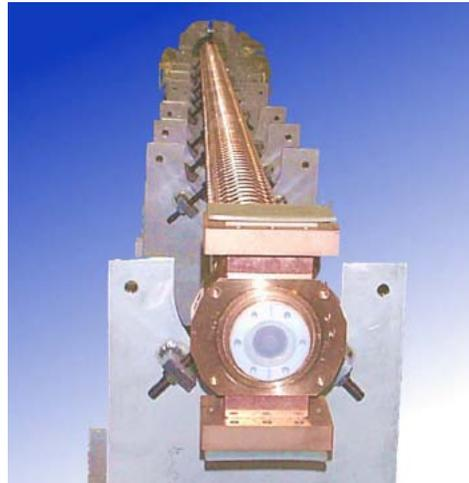
Figure 2: 5.2 m long S-band accelerating structures
