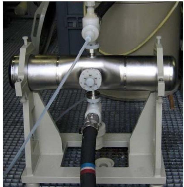
Figure 5: Prototype HWR during chemical preparation
