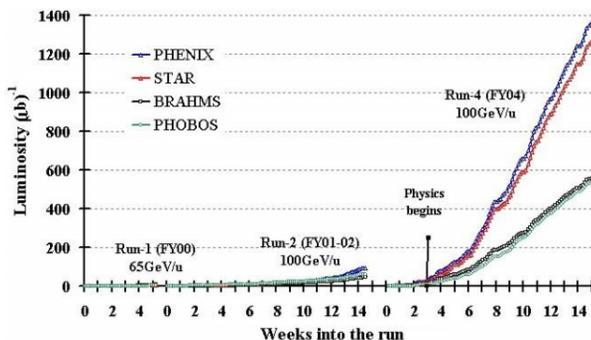
Figure 1: Integrated gold-gold luminosity delivered to the 4 RHIC experiments during Run-1, Run-2, and Run-4.
