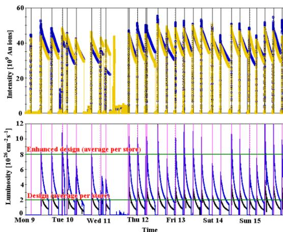
Figure 2: A week in February 2004. The upper part shows the beam intensities. The lower part depicts the instantaneous luminosities of a high luminosity (PHENIX), and a lower luminosity experiment (BRAHMS). The gap on Wednesday is due to 12 h of beam experiments.
